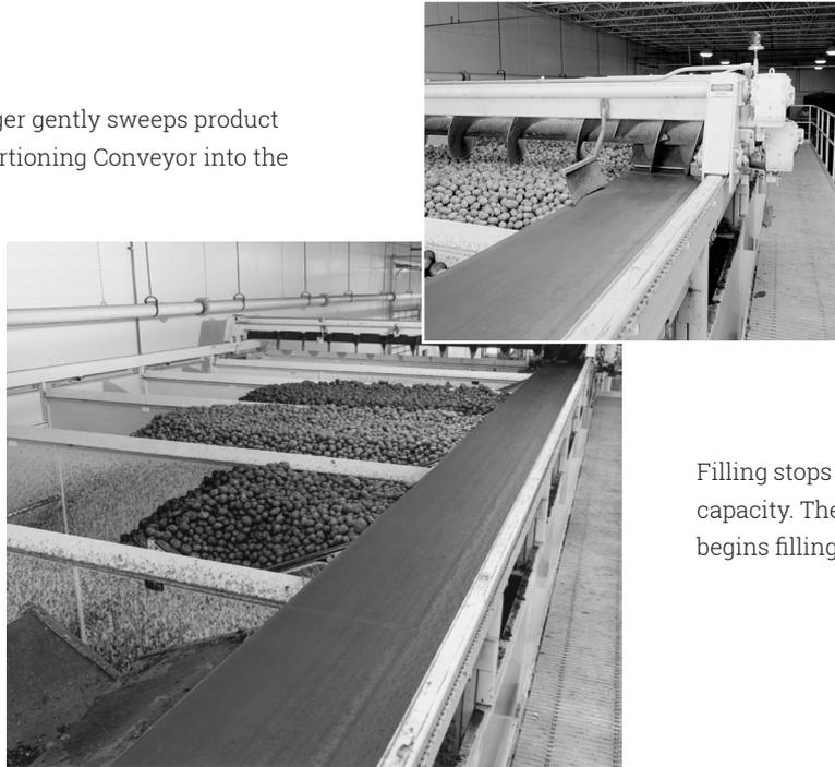
Filling stops automatically when the bin reaches capacity. The Bin Filling Auger levels product and begins filling the next preselected bin.
