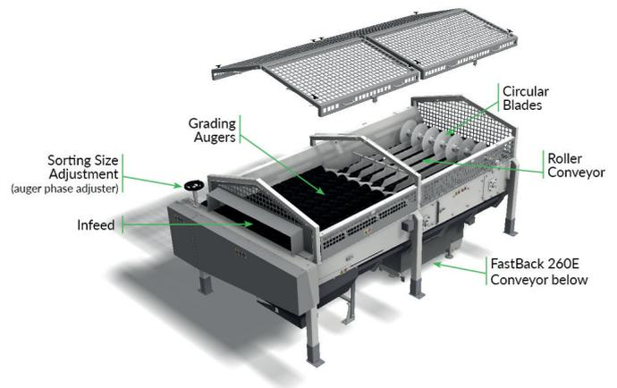
**Grading Augers - CLOSED PHASE (MINIMUM SIZE)**
