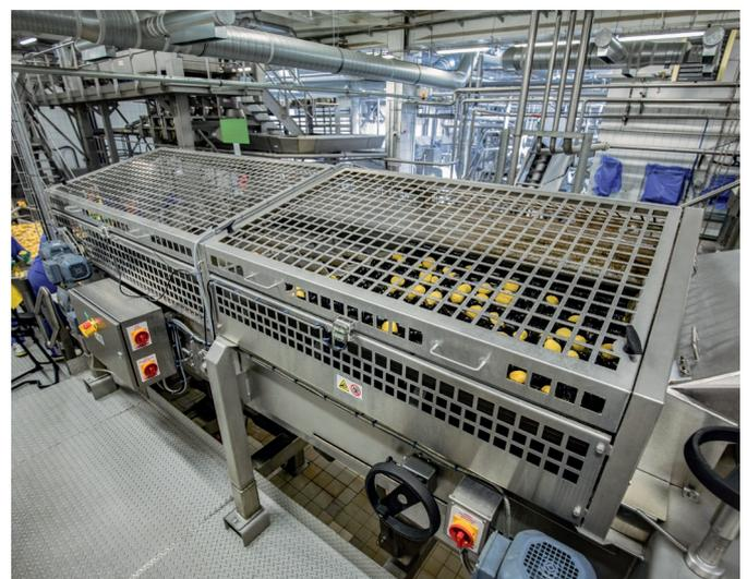
The full length grading area prevents small product from 'skipping' a short grading area and passing through. The grading size is easily adjusted at any time and features an adjustable reject for small potatoes (and small foreign objects, e.g. rocks etc)
