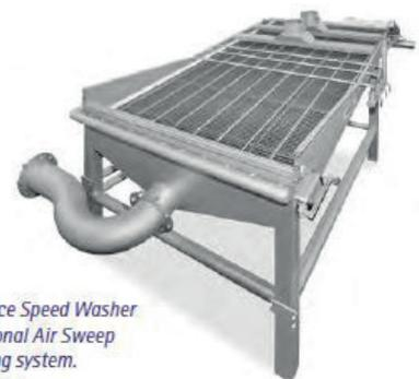
*Potato Slice Speed Washer with optional Air Sweep dewatering system.*
