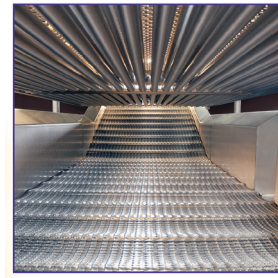
Heat transfer tubes and hood can be lifted clear of the fines removal conveyor to simplify cleaning.
