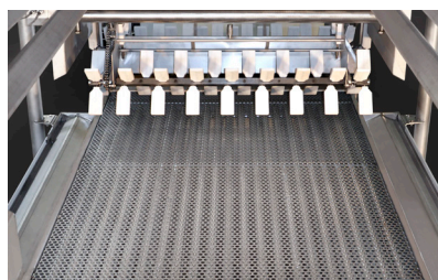
Chip-Stirr moves back and forth in the pan to uniformly fry potato slices.
