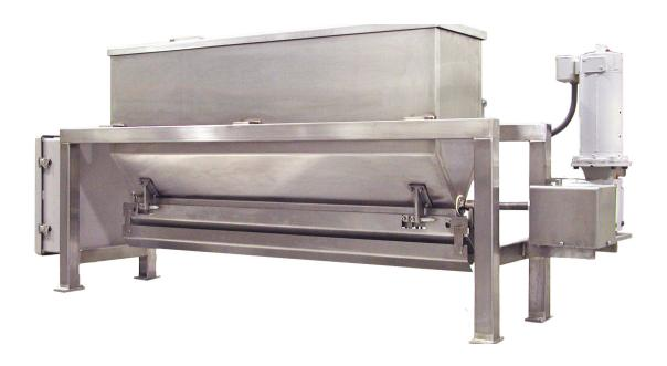
Metermaster evenly applies topical salt coatings without caking and clogging. A simple reciprocating distribution bar uniformly meters salt onto product passing beneath it. Metermaster requires no readjustment after cleaning, so coverage remains uniform from one production run to the next.
