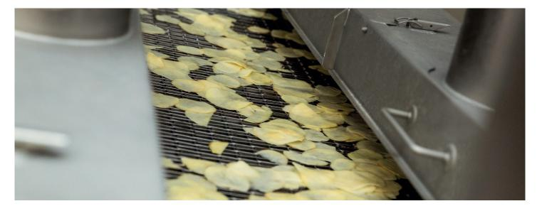
Producing two high velocity air curtains across the width of your conveyor or washer discharge, the Air Knife lifts and seperates product to remove surface water, starch and particles.
