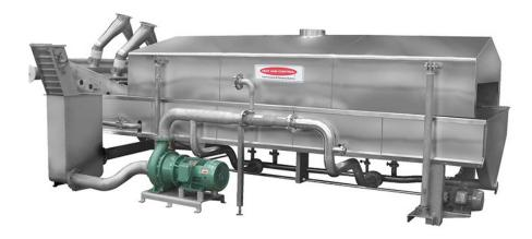
Multiple water jets in the bottom of the blancher tank force water up through the product pack. This spreads slices throughout the washer, separating them for greater surface exposure. Bottom-up water injection produces more uniform blanching than designs which inject water from the sides, compressing slices into a tight pack in the centre of the washer.
