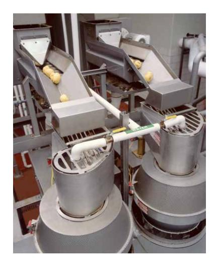
Rugged stainless steel washdown construction. Mounting hardware is optional.
