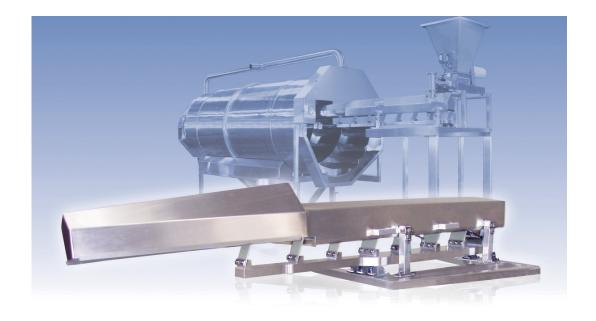
Spray Dynamics is a leader in providing the food industry with solutions for application of dry ingredients and other small particulates. The Scarf Plate Distributor optimises product coverage by providing an expanded, controlled curtain of particulates, either inside a coating drum or across a conveyor or belt.
