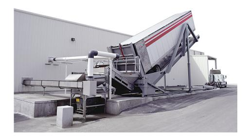
Single hinge design safely lifts trailers to empty product into a stationary transfer conveyor or flume system.
