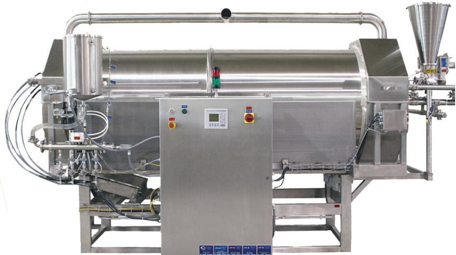
The Spray Dynamics two-stage coating system provides consistent, uniform application of liquid and dry coatings on extruded, baked, frozen, and fried products.
