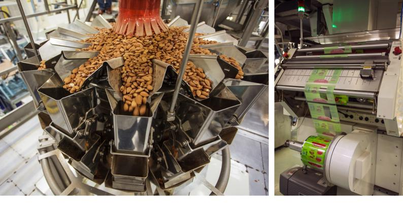
We have practically eliminated film waste, the Ishida simply stops when the film needs changing. With other machines, if the operator does not spot the need for a film change, then valuable product can be lost.
