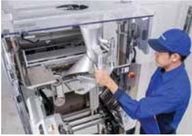
The new, open Inspira structure gives operators easy access to all important parts. Changing a forming tube has been made particularly simple, involving locating one corner on the support frame and swinging the former around the location pins until it locks into place.
