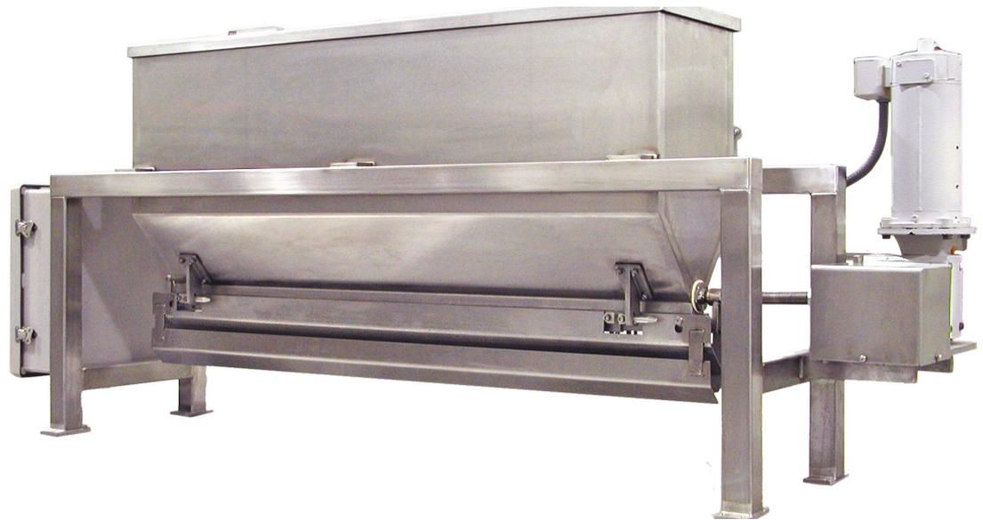
Metermaster evenly applies topical salt coatings without caking and clogging. A simple reciprocating distribution bar uniformly meters salt onto product passing beneath it. Metermaster requires no readjustment after cleaning, so coverage remains uniform from one production run to the next.
