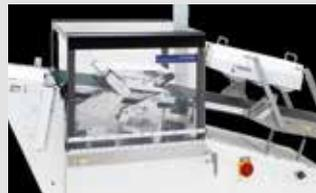
Ishida TSC-RS for high-speed and accurate detection of leaking packs and integrated bagmaker control.
