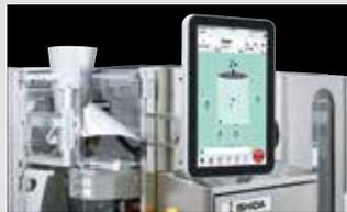
The equipment is very straightforward to control via a user-friendly icon-based interface similar to a smartphone. The intuitive, 15.3-inch screen can be customised by users.
